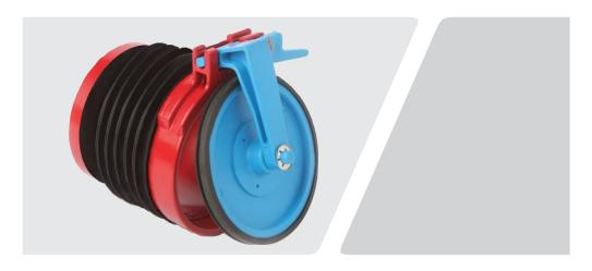
To prevent foul water flowing back from the blocked sewerage system to flood the property from the inside via toilets, plug holes and waste pipes. These unique and patented Retrofit Non-Return Valves can be simply pushed in to the existing pipework, whether plastic or clay, at the property's inspection chamber. The valves can be fitted in minutes and do not require any specialist expertise or equipment.
